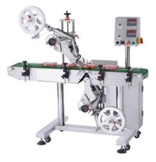
We provide highly efficient labeling machine that provides labeling on top and bottom surface at one time. It is a cost effective automatic top labeling machine which has powerful servo head and removes many bells and whistles. It has speed of over 100 per minute for labelling. This machine is equipped with label dispense head that provides accurate output.
