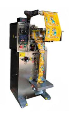
This granules nuts packaging machine adopts correcting system controlled by microcomputer, owing to a response signal is handle and set pass through microcomputer, It can accomplish whole set to synchronization, sack length, position fixing, voluntarily follow the tracks of light-mark and voluntarily diagnose trouble and show to screen.
