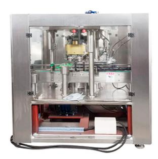
This kind of machine is mainly used for easy pull cans made of tinplate, aluminum alloy can or PET cans capper, It is very good ideal facility for canned food plant, beverage plant, wine plant, etc. It has automatic stop device in case of problems like no cap for can, no can no cap, can block and other problems.
