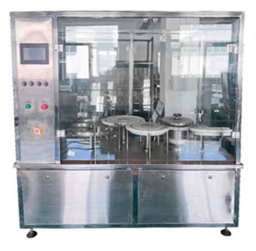
This machine is suitable for special-shaped tubular glass bottles with diameter of 22, 24, 30mm, which can be customized according to different bottle sizes. Linkage line design, can achieve aseptic isolation operation, positioning plate adopts precision protractor, stable and reliable performance, machine speed stepless adjustable, suitable for different product filling requirements.
