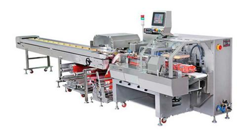
The bun packaging machine also belongs to the down film type packaging machine, which is designed for the high product, secondary package, group package, or family package. This type of frozen food packaging equipment controlled by 5 servo motors can pack multi-bags.
