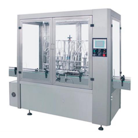
ALF Automatic Volumetric filling machine for the application of light liquid filling into plastic or glass bottles. The machine is composed by a conveyor, SS316L volumetric piston pump, top-bottom filling nozzles, liquid buffer tank and bottle indexing system. The bottle loading/unloading through loading/unloading turntable or directly from an production line.
