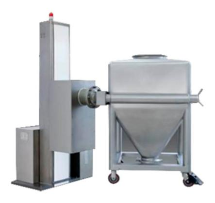
Our HLT post bin blender is extensively used for mixing dry powder with another dry powder, or dry powder with grain in a variety of solid product preparation within the pharmaceutical industry. This mixer can be equipped with hoppers available in various specifications, and it is suitable for mixing a variety of pharmaceutical products and batches, based on technological requirements from large and medium sized companies. Multiple processes can be achieved using a single machine.
