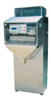
The machine consists of feed hopper, vibratory feeder, weighing device, weighting hopper, door opening mechanism etc.
