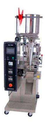
This vertical form fill seal machine is an electricity driven type packing machine, with compact and dedicate design by Techier Industry, catering for owner operated SOHO, small business and medium enterprise.
