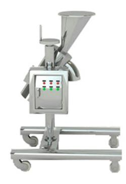
KZL High speed Granulator Series are widely used in pharmaceuticals, chemical industry, and foodstuffs with good stuffs with good effect. It's designed reasonably with filter net, shaft. It cans gring a block of material that is easy to smash. The specialized friction filter cans gring solid particles on a big block according to centrifugal force principle. It can replace sway granule machine.
