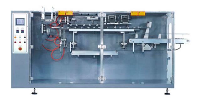
This Bag Filling and Closing Machine is flexible enough for automatically packing chemical industry, food, medicine products. To work with different filling equipment's, it can pack granular, powder, paste or liquid etc.
