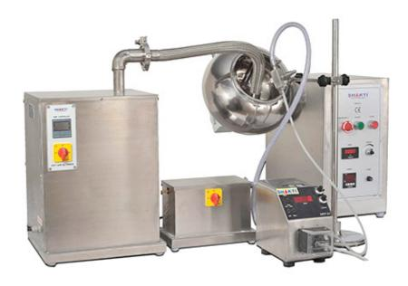
Coating With Peristaltic Pump, Spraying & Drying System: The Coating pan is used to produce uniform coating on tablets with the help of Baffles inside of pan. This can be mounting on the universal Gearing and as a result different tilting angle can be set up to 45 Degree.
