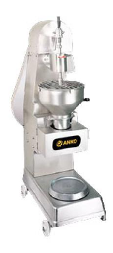
By putting paste materials such as meat paste or fish paste into the hopper, the FMB-60 can make ball-shaped foods automatically. It is equipped with a rotary round platform for putting a bowl of water to collect final products and prevent them from sticking.
