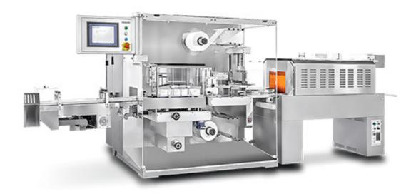
HB 40S is an automatic stretch banding and shrink wrapping machine for cartons and blisters optimal for high speed operation, producing 40 bundles per minute through servo driven technology. High quality seal is provided for stretching resistance and if shrink-wrapping is required for certain products, a shrink tunnel is installed as an integral part of the machine.
