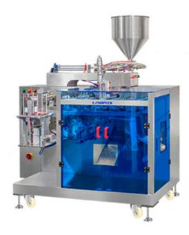
Automatic Doypack Laundry Detergent Stand Up Premade Pouch Packing Machine, suitable for the liquid or the semi-fluid materials packaging, such as detergent, soy sauce, vinegar, jice, beverage, jam, sauce, paint etc.
