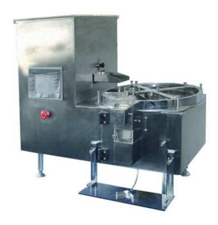
Mini electronic counting and filling machine CCD sensitization technology, PLC control, human and machine interface operating system count automatically, put bottle by manual and fill medicine automatically, high differentiate rate, fast responding speed, count accurately, it is no need to change mould when change the type of medicine. And it can set the filling quantity in the touch screen.
