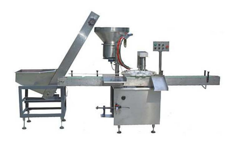
This machine is suitable for the capping of wide mouth bottles.
