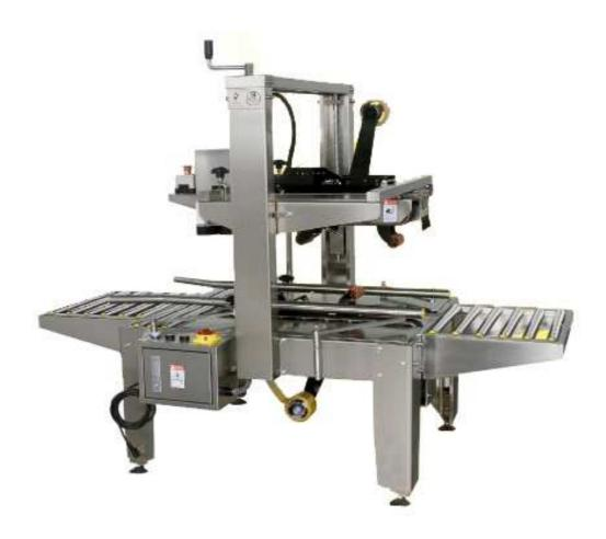
Carton sealers are case equipment that seals the top or bottom of a case with tape or glue. Typically, the minor corrugated flaps are kicked and plowed closed as the cases are transferred. As the cases enter the compression section, the major flaps of the carton are closed and a hot-melt adhesive is applied.
