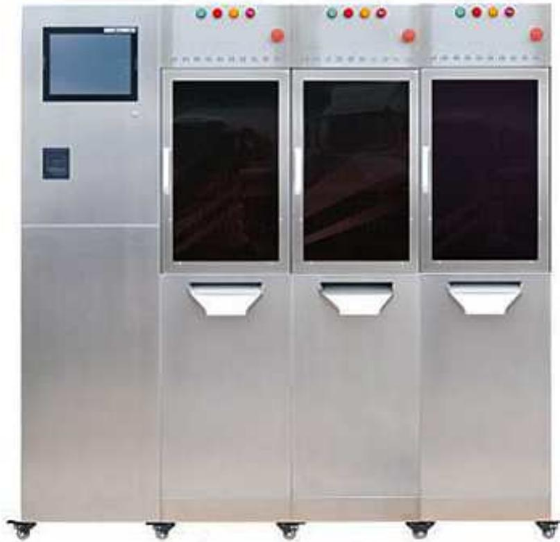
CMC series could classify every capsule weight single by single with high precision. Capsules will be divided into qualified and unqualified section according to the standards set in advance and a report of data statistics will be printed out simultaneously. This machine could weigh the risk capsules one by one, even the capsule number is large, and separate the good and bad ones into different area. Pharmaceutical plants could benefit from this to lower the cost and improve the quality.
