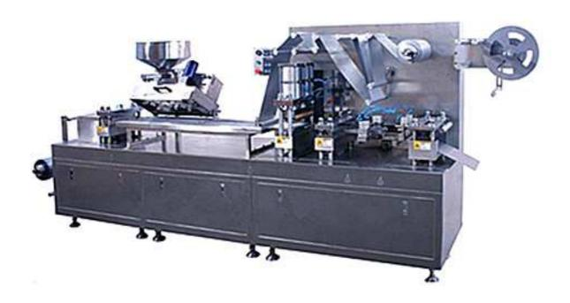
The blister packing machine is special for pharmaceutical, food, chemical industrial usage. It has the function of packaging, detecting, rejection. It adopted PLC control system, touch screen interface, frequency converter system, which make the machine automatic running more stable and enhanced the machine life time. The machine can use ALU PVC, ALU ALU, PVC PAPER material for blister packaging. It meet GMP standard.
