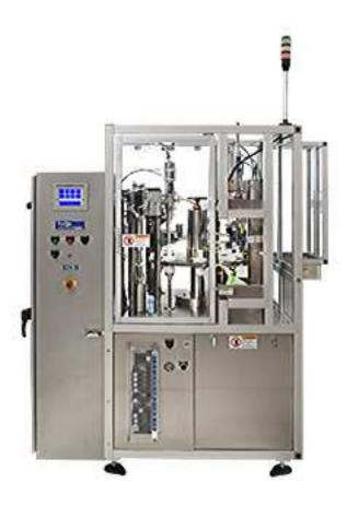
The RS8 syringe filler with speeds to 60 syringes per minute has a compact 8 station dial and will fill and close a variety of syringe styles.
