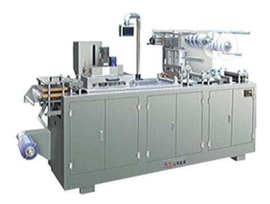
DPP-250F Flat Panel Automatic Blister Packaging Machine collects optical-mechanical-electrical-pneumatical as integration, and it's controlled by programable PLC Human-machine interface system. It is widely used in packaging industry of pharmaceutical, foodstuff, electron, medicine equipment and metals products.
