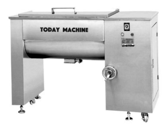
Used in the mixing of solid-solid (ie powder and powder) solid-paste (ie powder and cement) for pesticides, veterinary drugs, food, chemicals, biology, aquaculture, ceramics, refractoriness, plastics, compound fertilizers, etc. It is also specially adapted to the mixing of viscous materials.
