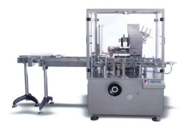
Automatic Bottle Cartoning Machine for bottle is suitable for automatic feeding bottle (round, square bottle) into carton (either for blister or bottle). On line bottle unscramble and feeding, leaflet fold(1-4 folds) and feeding, leaflet detecting, canton opening and forming, products and leaflet pushing into carton, printing batch number, sealing carton with tuck-in or hot melt glue device. Automatically reject lacking of leaflet or product and finished product out.
