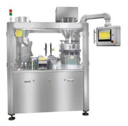
The NJP4200 automatic capsule filling machine is a kind of intermittent motion capsule filling equipment designed with multiple tamping stations and stable performance. The pharmaceutical machinery is capable of completing capsule feeding, separation, filling, removal of defective capsule, locking, and discharging, automatically.
