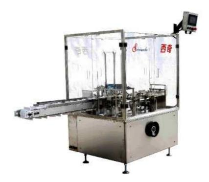
The cartoning machine, is a packaging machine that can put the products into the carton automatically: open, load, close and seal cartons. Cartoning machines are widely used for packaging bottled foodstuffs, confectionery, medicine, cosmetics, etc., and can vary based on the scale of business.
