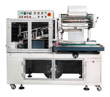
Fully Auto L-sealer, LSA-504 is adjusted easily for size change. It can run multiple package to help promotional purpose. The sealing cutter is installed safety & alarm system to protect worker.
