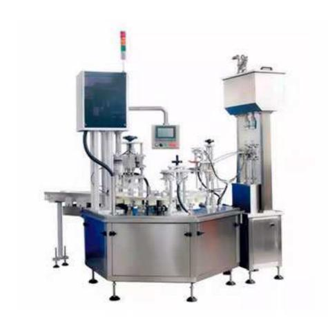
This machine adopts hexagonal turntable multi-station mode, which is suitable for small daily chemical products, cosmetic and other industries with multiple varieties, multi-process and relatively high production capacity.
