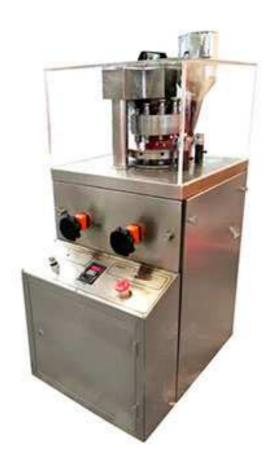
ZP-7B vitamin pill press machine is single pressing type, capable of automatically rotary pressing raw granular into tablets. The max. Diameter of tablet can be 20mm.
