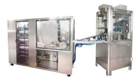
As a market leader in liquid-fill technology, we have taken extra care to ensure proper filling of liquids. The NSF capsule sealing machine seals the cap and the body of the capsule at high speed.
