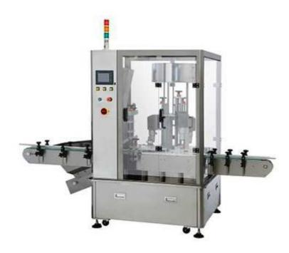
High Speed Rotary Capping Machine CR-635S is high speed rotary capping system easy to get 80 BPM capacity.
