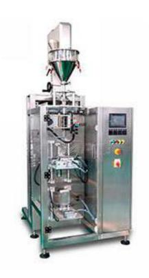
This machine completes the whole packing procedure of measuring, loading materials, bagging, date printing, charging (exhausting) and products transporting automatically as well as counting. can be used in powder and granular material. like milk powder, Albumen powder, solid drink, white sugar, dextrose, coffee powder, and so on.
