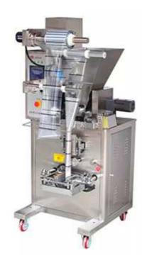
HXL-F Series Automatic powder packaging machine adopts microcomputer to control the length of the bag, copulate photo electric and helix-falling. It can automatically finish metering, making bags, counting, filling, sealing, coding and cutting and printing batch number. It is fits for 100-300MU powder.
