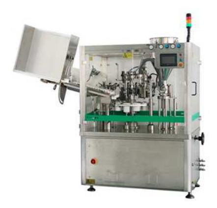
Rotary filling and sealing machine can fill and seal plastic pipes and plastic aluminum laminated pipes. Widely used in cosmetics, medicine, lubricants, adhesives, shoe polish and food industries. Rotary filling and sealing machine fills and seals aluminum tubes. It can smoothly and accurately inject all kinds of paste, viscosity fluid and other materials into the aluminum tube. Complete the folding and sealing, batch number and production date.
