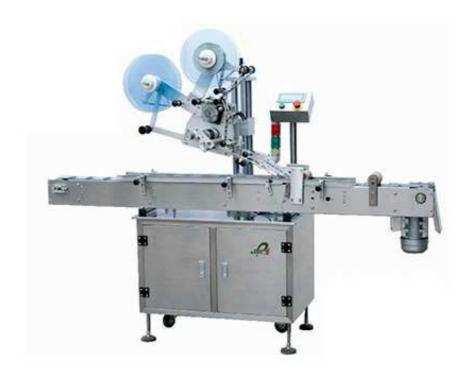
Top labeling machine is suitable for all kinds regular and regular containers, flat surface, such as, pouch, bag, carton, box as so on
