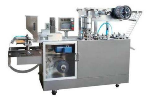
Blister Packing Machine DPP-140 is specially designed for hospital dosage room, laboratory institute, health care product, middle-small pharmacy factory, and featured by compact machine body, easy operation, multi-function, stroke adjustable, long durability etc. It is suitable for the Alu-PVC package of medicine, food, electric parts etc.
