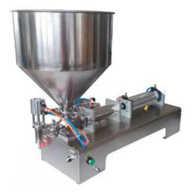
The small butter filler machine filling volume and filling speed can be adjusted, suitable for filling liquids, paste, cream etc in industries such as chemical, food, daily chemical, pharmaceuticals.
