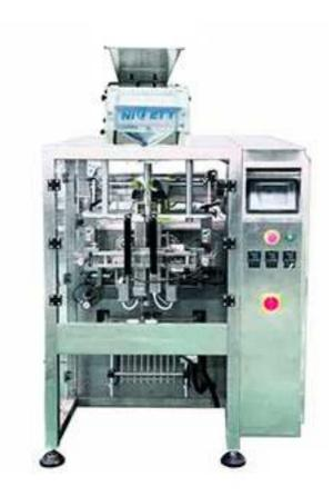
The single-file equipment counts and fills capsules, soft gels, normal tablets, special shape tablets, coating tablets, pills and most solid granules in small bags. Counts by infrared and sensor that doesn't wear or break the product and is compatible with all kinds of materials. Can accomplish bag forming, counting, filling, bag sealing and printing at the same time.
