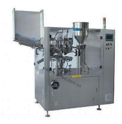
Automatic Tube Filling and Sealing Machine applies for production in cosmetic, light industry (daily use industrial goods), pharmaceutical and food industry, etc. It can fill material such as grease, ointment, gel and sticky fluid extract into tube, then seal the tube end, stamp number and discharge finished product.
