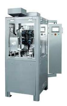
GTI - C600 Automatic Capsule Filling Machine processes the products for optimal productivity up to 40,000 capsules per hour, featuring low-maintenance operation, minimal downtime, and overall dependable production. Filling of pellets is available. With different specifications of mould, No. 00 to No. 5 hard capsules and safety capsules A, B, C, D, E can be filled. Both slow-released pellets fill and mixed fill with powder and pellets can be realized.
