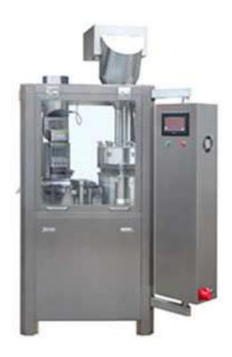
The machine can fill powder, granules or pieces of material into hollow capsules. It adopts hole plug type filling, intermittent operation, frequency conversion speed regulation. The production process is in full compliance with GMP specifications.
