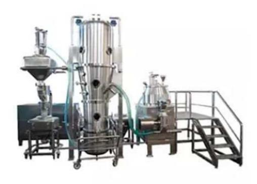
This is an closed-wide automatic granulating production line, it includes rapid mixer granulator, fluid bed dryer, screener, and the grinding granulator to get high quality dry granules for good preparation processing.
