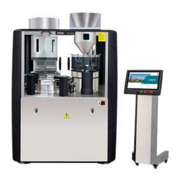
The whole machine supports modular design, can quickly clean and replace the mould, equipped with a leading IPC operator interface; Has a quick and convenient modular filling compaction mechanism; With a brush blowing air cleaning agent position; All-round seal capsules, simple and lightweight without damaging the capsule.
