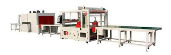
GH-6030AF Fully-auto Horizontal Double Side Sealer which is developed for special big items adopts advanced high speed double-side sealing technology. It has up & down single film rollers. The film is in sync with the items. While the items are going forward, the side sealing system starts to seal and cut the up & down film that keeps good sealing;
