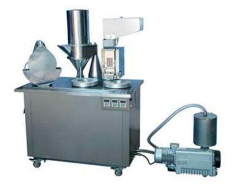
The machine is an intermittent motion and hole plate type semiautomatic capsule filling equipment.
