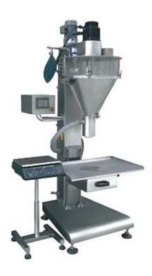
ZH-1B3 semi-automatic powder bagging machine is typically designed to pack corrosive materials, like agriculture pesticide. Its packing weight ranges 10 g to 5000 g and packaging rate is 10 to 50 bags in one minute. The hopper volume is 50L. Such powder filling machine adopts the weighing feedback track filling type.
