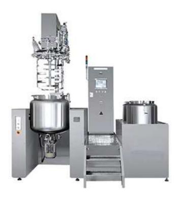
Hydraulic Emulsifying Mixer With Bottom Homogenizer is a high quality and efficient mixing equipment for cosmetic production. The bottom homogenizer is suitable to dealing large volume and high viscosity material with strong shearing.
