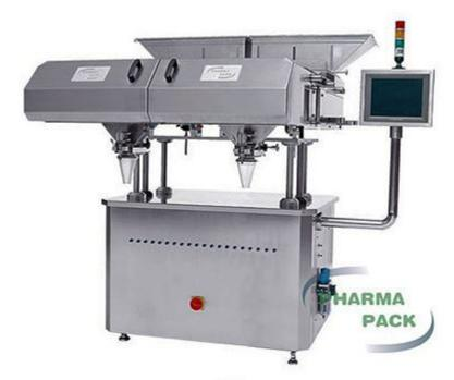
The counter PP-16 is a reliable, high performance machine, designed in conformance with current and proposed GMPs. Having a small footprint, they are effective in maintaining the integrity of a clean room environment. Few change parts are needed for different container sizes (only the nozzle). All product contact parts are made of type 316 stainless steel. And all contact parts can be easily disassembled for cleaning.
