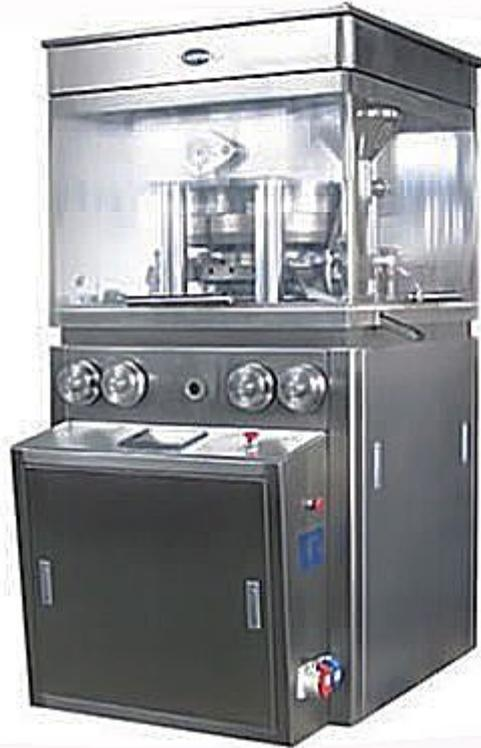
ZP27 double sided rotary tablet press is a kind of punching automatic tablet press. It can press granular raw materials into tablets with different shapes, double colors and letters on both sides. It is mainly used in manufacturing piece prescription in pharmaceutical, chemical, food and electronics industries. When manufacturing double color pieces, it only needs replacing components and adding powder absorbing apparatus, which greatly lowers the cost and increases profit.
