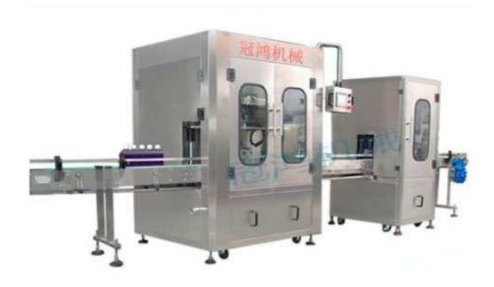
Automatic filling machines is special filling for liquid items, with 1 heads filling, would reach the speed 1800 bottles per hour for 500ml bottle. it is welcome by customer and customer offer it a name as smart machine, as it reach accurate capacity and also would automatic cleaning funcation as well.
